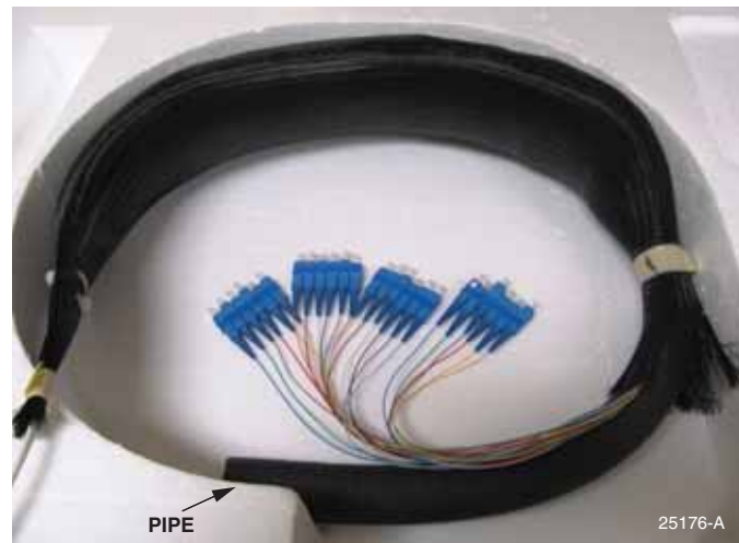
Figure 44. Removing Pipes from 900 mm Fanout Assemblies
